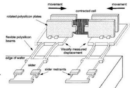
Figure 10. MEMS device for detecting cardiac forces<sup>[37]</sup>.
