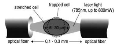
Figure 6. Optical Stretcher system, developed by Guck et al.<sup>[17]</sup>. Two diametrically opposed laser beams confine the cell in a two dimensional potential well. By narrowing the well, the cell is squeezed.
