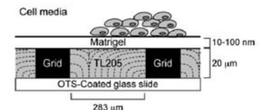
Figure 7. Liquid crystal culture device developed by Palecek et al.<sup>[32]</sup>. The TL205 is liquid crystalline material, which displays changes in colour depending on deformation.
