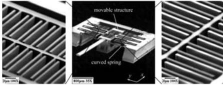
Figure 11. MEMS capacitive cellular force sensor<sup>[38]</sup>.
