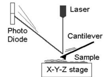
Figure 5. AFM Schematic<sup>[16]</sup>. A laser beam is reflected off a cantilever. As the cantilever is rastered across a sample, it deflects based on the topography, shifting the reflected beam on the photodiode.
