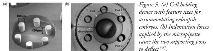
Figure 9. (a) Cell holding device with feature sizes for accommodating zebrafish embryos. (b) Indentation forces applied by the micropipette cause the two supporting posts to deflect<sup>[35]</sup>.
