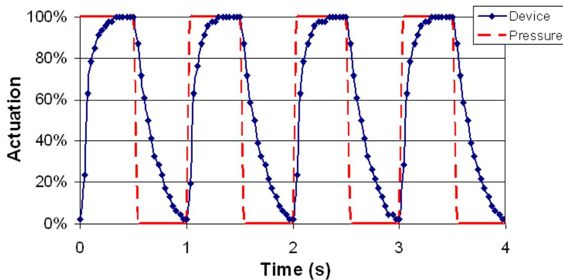
**Figure S2.** Dynamic characterization of device actuation in response to a 1 Hz cyclically applied square pressure waveform. Results obtained by video microscopy and subsequent image analysis of culture film deflection.
