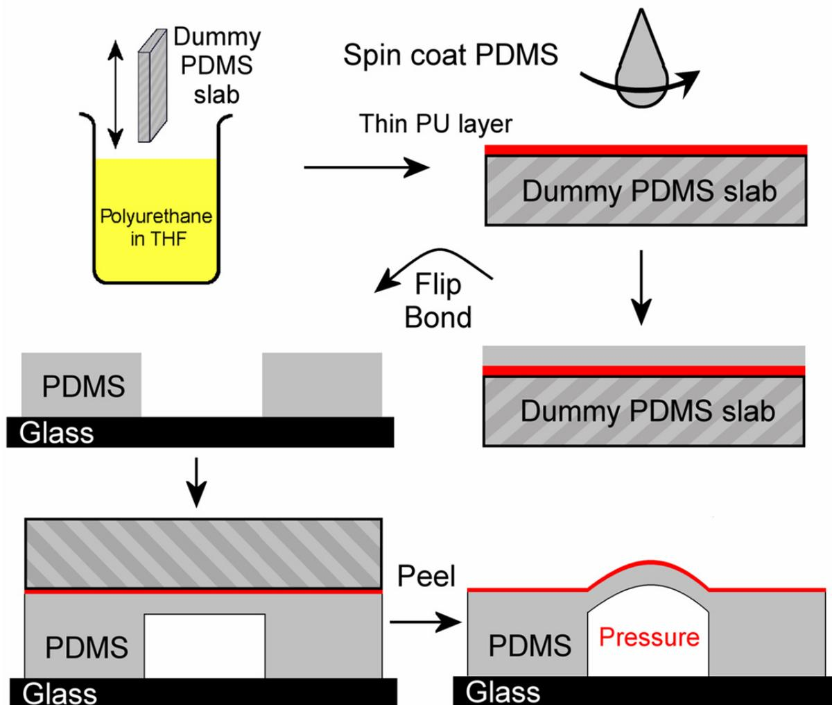
**Figure S1.** Fabrication process for the composite culture films and mechanical stimulation system.
